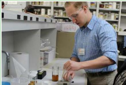
John Wulterkens (Technical Service Engineer) showed his group how to troubleshoot VpCI®-377 application problems with a refractometer. Measuring product solution concentration with a refractometer can help the distributor decide if the customer needs a higher concentration of the fluid to prevent rust, or if contamination (indicated by a falsely high concentration reading on the refractometer) is causing product performance problems.
