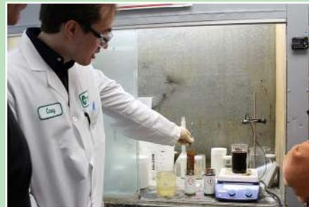
Casey Heurung (Technical Service Engineer) demonstrated rust removal and the benefits of heating VpCI®-422 to speed up the process. He also showed how unheated VpCI®-422 removes rust much more slowly, and how VpCI®-426 is a quicker rust removal alternative in situations where it would be difficult to heat VpCI®-422.
